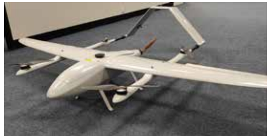
Baby Shark long endurance VTOL drone used for agricultural mapping
